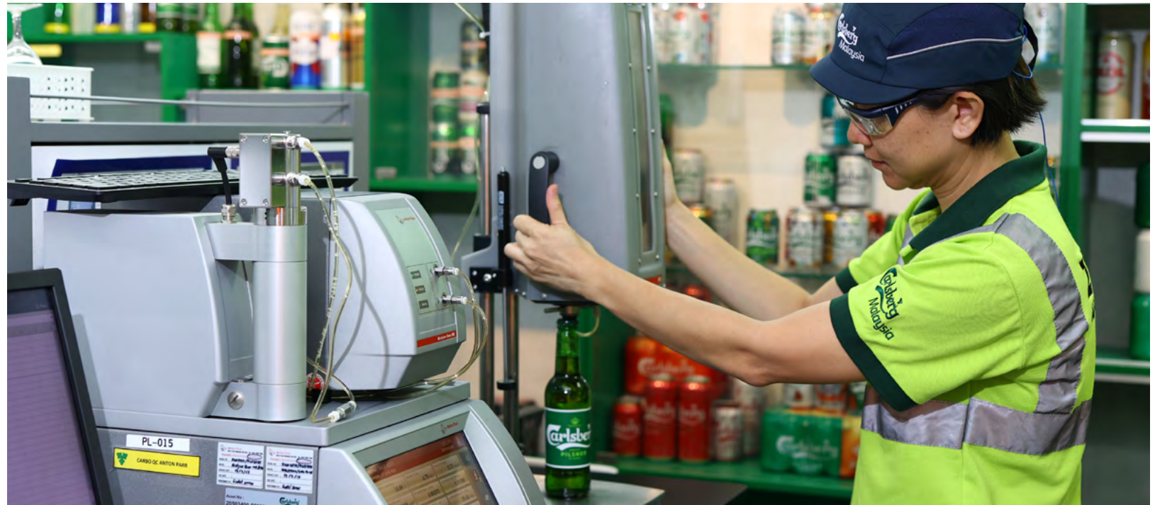
A quality control process being undertaken to test alcohol quality, where testing is conducted on alcohol percentage, CO 2 levels, degree of fermentation and °P (Plato gravity scale).
